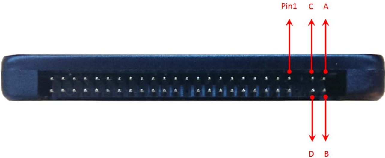
Figure 3 : The connectors of 2.5" PATA SSD
