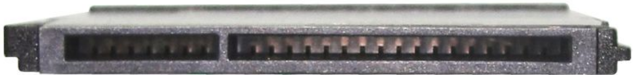
Figure 3: SATA 7-pin (data) + 17-pin (power)
