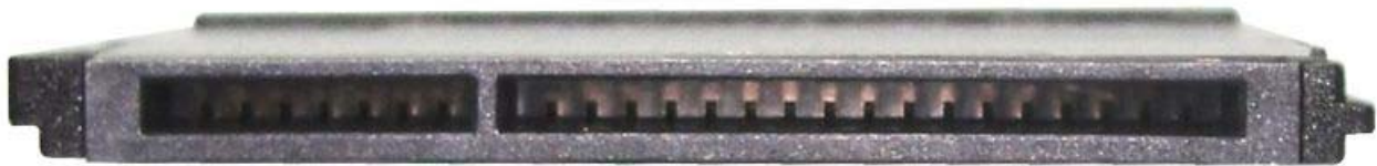
Figure 3: SATA 7-pin (data) + 17-pin (power)
